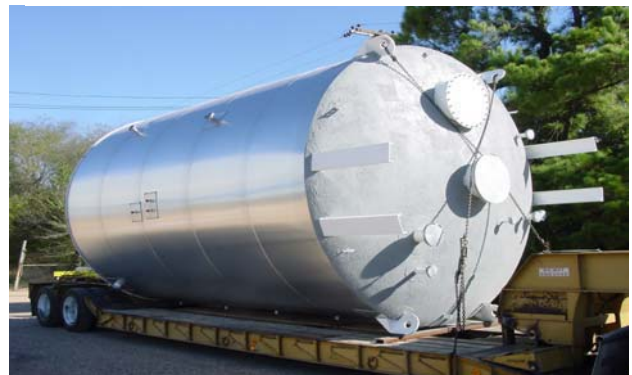
15,000 gallon heated and insulated chemical tank with top agitator support structure.
