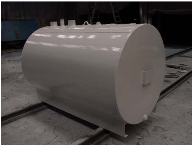
550 gallon UL142 double wall skid tank awaiting accessories installation.
