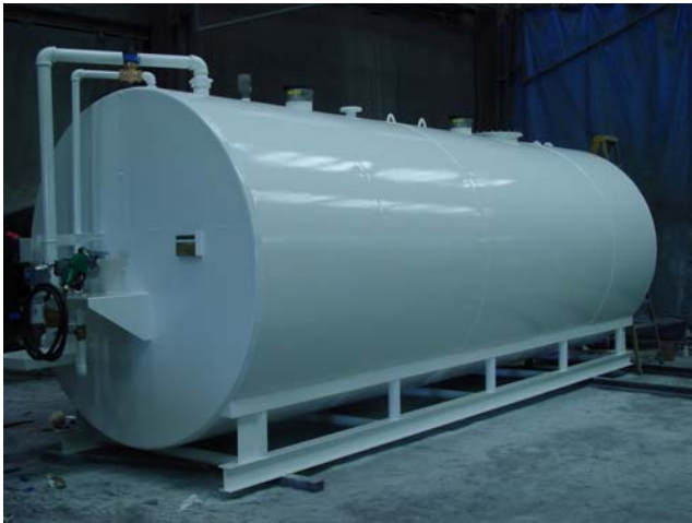
8,000 gallon UL142 double wall fuel skid tank with ground fill and dispensing system.
