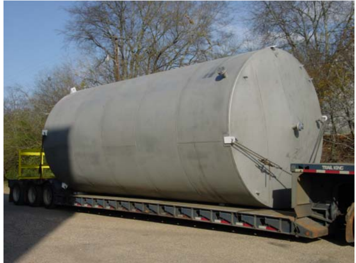
20,000 gallon stainless steel water tank.
